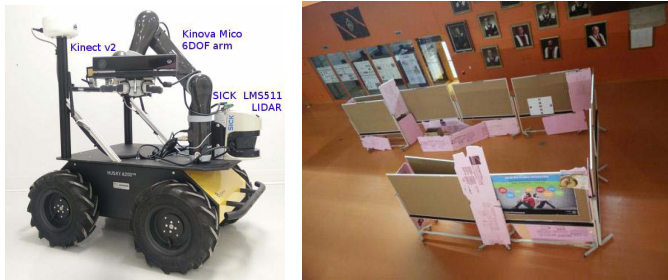
Fig. 17. Left: Husky robot used in our experiments with the robotic arm, depth sensor, and laser range scanner. All other sensors seen are not used. Right: indoor structure being inspected.
