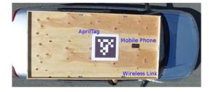
Fig. 4. Experimental setup showing the required equipment on the car. In practice the mobile phone could also be held inside the car as long as GPS reception is still good.
