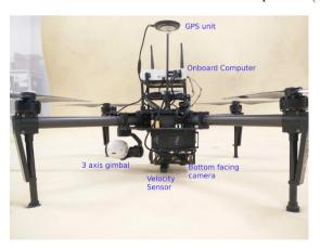
Fig. 3. The M100 quadcopter. Note that all side facing cameras of the Guidance module were removed and the down facing BlueFox camera sits behind the bottom guidance sensor.
