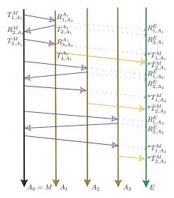
Fig. 1: Simultaneous ranging and synchronization protocol example with 4 anchors  $A_i$ , i = 0, ..., 3 and one tag E.
