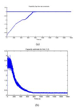
Fig. 3. (a) Trajectories of the routing constraint values  $g_i^{\phi}(a_i^{\phi}[k], \mathbf{r}_{i.}^{\phi}[k])$ . Note that the communication constraints are essentially always satisfied during deployment. (b) Sample trajectory of the capacity estimates (19) for the link (1,2), with  $\gamma = 0.2$ .
