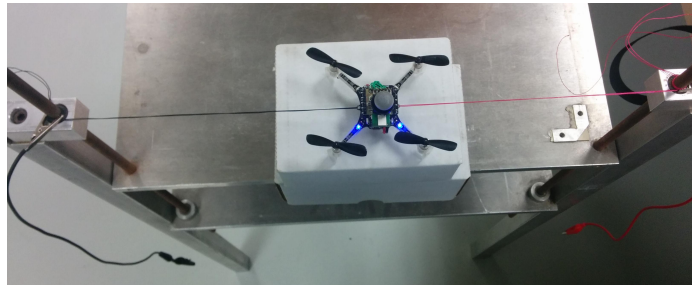
Figure 4.2.1: Pitch angle calibration rig.
